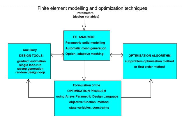
Developing of parametric FE models in mechanical engineering proved to be very useful for comparative analyses and design procedures.
